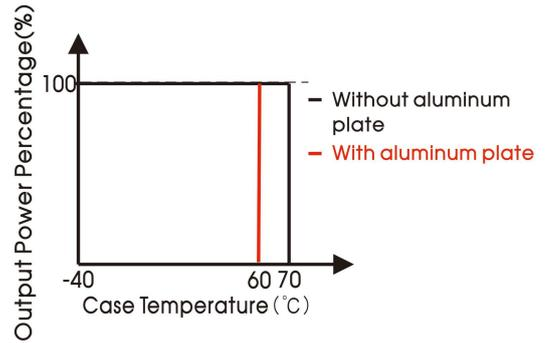
Note: 1. With an AC input voltage between 85 -100VAC and a DC input between 120-140VDC the output power must be derated as per the temperature derating curves;
