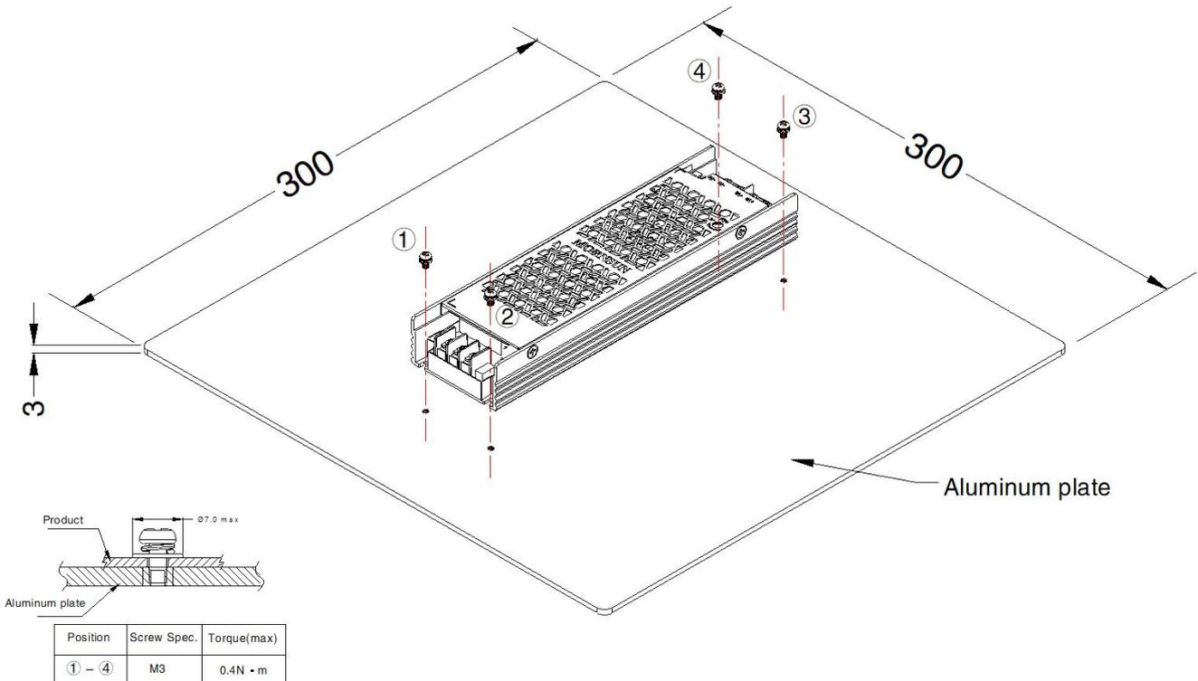
Note: 1. In order to meet the "Derating Curve", the product testing must be installed onto an aluminum plate. The size of the suggested aluminum plate is shown as above. And for optimizing thermal performance, it is necessary to apply thermal grease on the bottom of the product.
